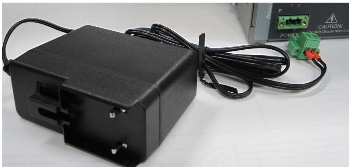
Figure 10 AMU-RTS power supply
