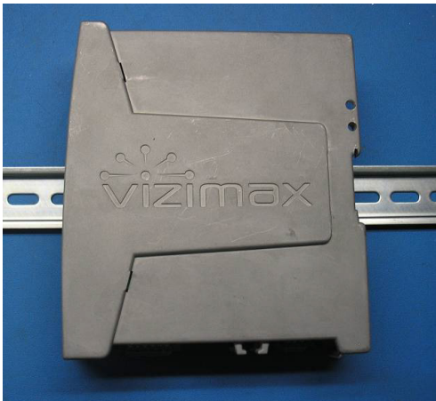
Figure 3 STCM Panel mount with optional adapter (RWA AA0000)
