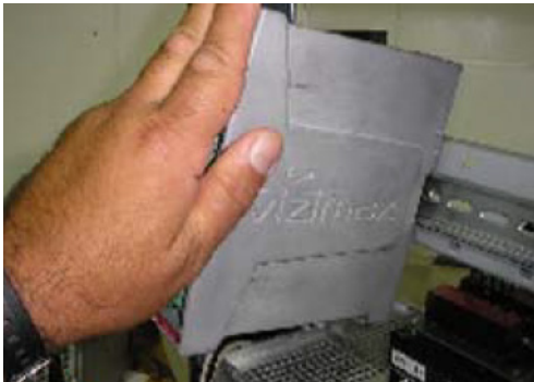
Figure 2 STCM DIN rail mounting
